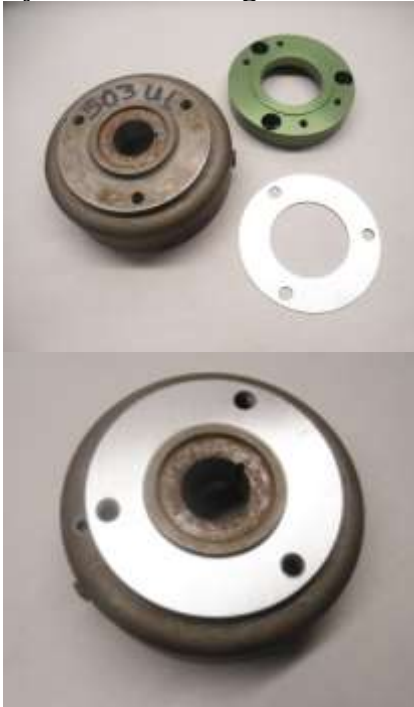
Shim plate on flywheel (Picture 2)
